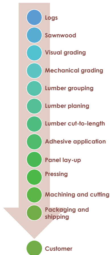
Figure 4.2. CLT production process
